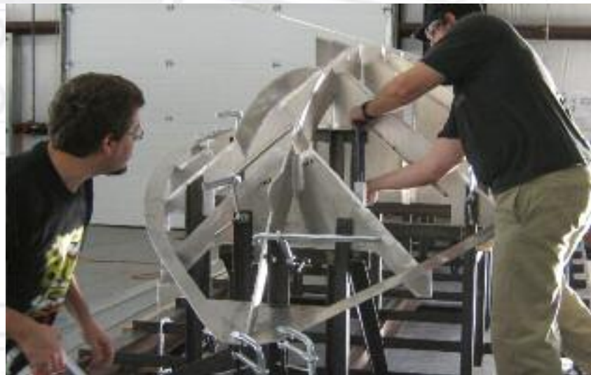
Keelson and Longitudinal Girder Construction
