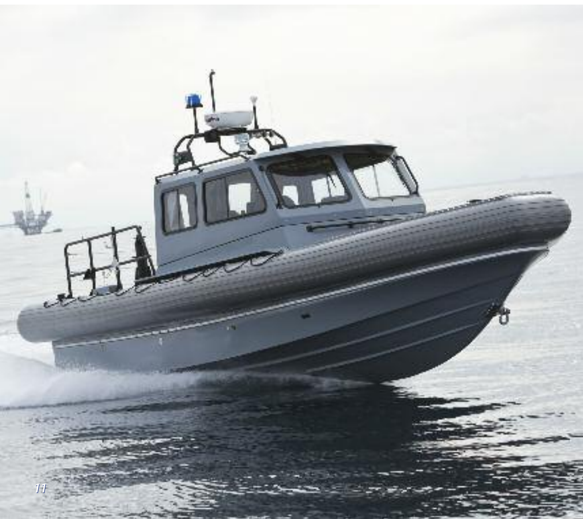
This boat is an upgraded version of our 11m with added options including Shock Mitigation seats for the crew
