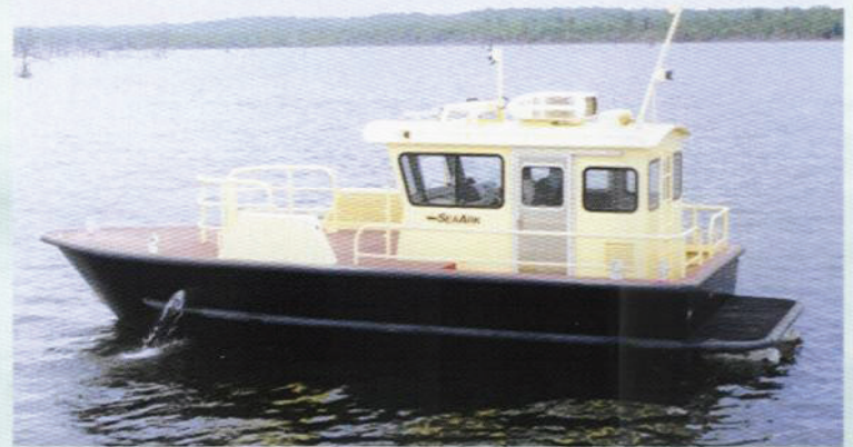
3010 Enforcer, with extended survey cabin, twin diesel jet, flush fwd deck, mid hull rubrails, and custom paint.
