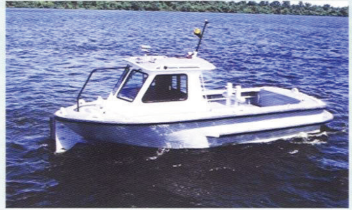
2610 Enforcer-Line Handler with forward push knee, 2-man cabin, heavy-duty rub rails, heavy-duty tow bitt and a single diesel inboard.
