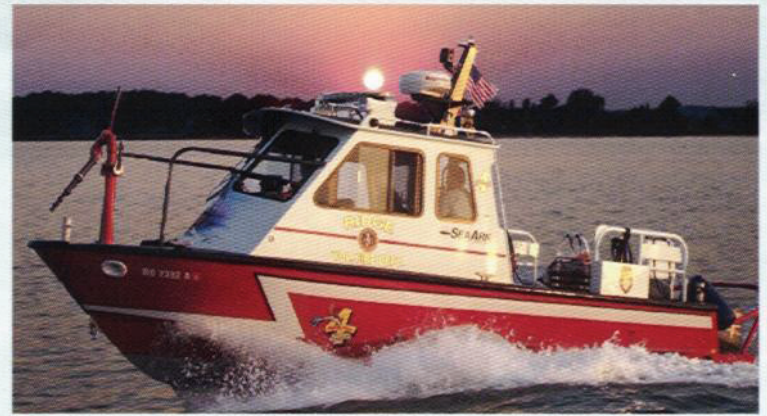
2610 Enforcer, Fire/Rescue, optional 4-man cabin, flush deck, 500 GPM internal fire system, bow docking lights, and twin outboards with protection bar.
