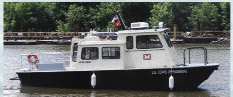
3512 Enforcer, crew cabin configuration, bow and stern safety rails, roof top AC, and I/O protection bar.
