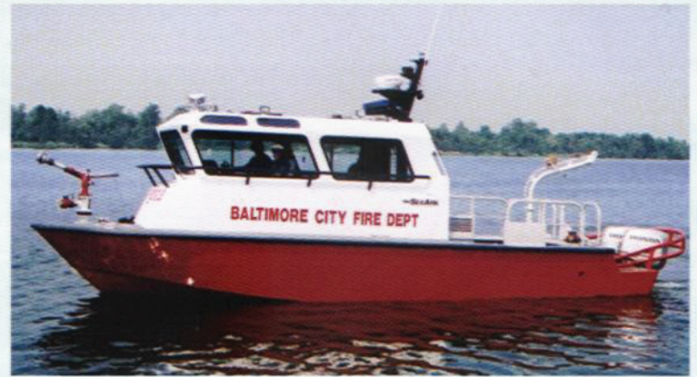
3010 Enforcer, Fire/Rescue, 1500 GPM fire system, integrated engine mounting platform, rescue davit, and extended treatment cabin.
