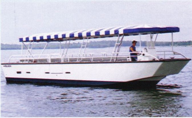
3510 Enforcer, Excursion configuration, with twin outboards, forward console, side loading doors, full canopy, and stadium seating.
