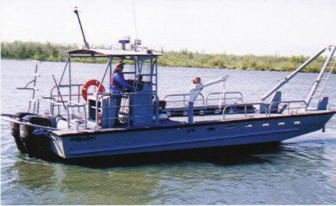
3512 Enforcer, open workboat configuration, bow door, "A" frame, elevated aft console and t-top.
