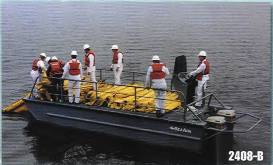
2408-B Transporter with optional flush deck, side safety rails, boom tow bar and bow roller.
