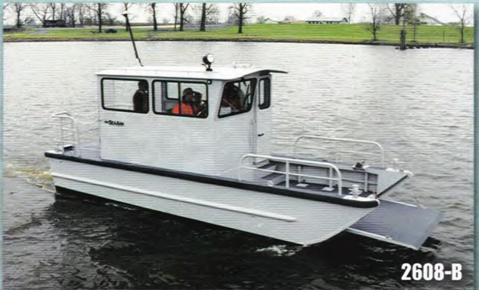
2608-B Transporter with stern drive propulsion, optional extended crew cabin and optional bow ramp.
