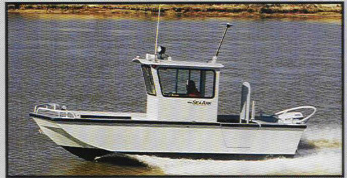
21' Roustabout with pilot house, tow post arrangement and dive door.
