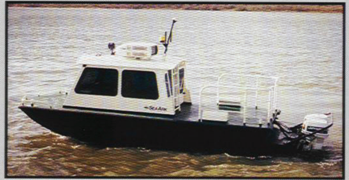
23' Little Giant with optional 10' survey cabin, air conditioner, emergency strobe light, aft wall with door, roof access ladder, flush aft deck, 3-tier safety railing and O/B platform with protection bar.
