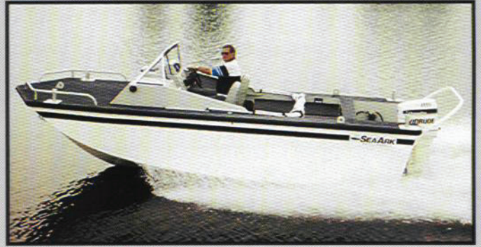
19' Roustabout with optional lifting eyes, convertible top and outboard protection bar.
