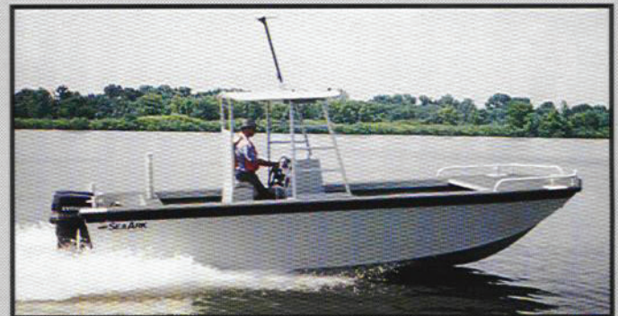
23' Roustabout with optional heavy-duty "A" top, single tow post and operator safety screen.
